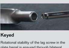
Rotational stability of the lag screw in the plate barrel is ensured through bilateral flattening of the shaft of the lag screw to match the inside of the hip plate barrel.
